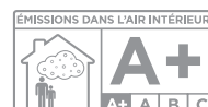
Statement on level of emission of volatile substances in indoor air posing a toxic threat during inhaling - on a scale from A+ (very low-emission) to C (high-emission)
